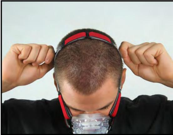
The strap on top of your head can be tightened or loosened by adjusting the Tri-Glide connection. Adjustments to this top strap connection can be made by pulling the Velcro straps up and then pulling outward.
